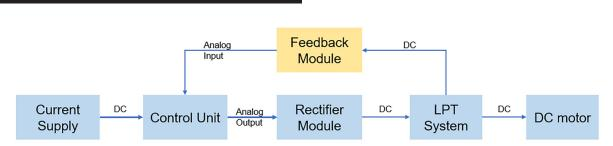
Fig. 7. Control strategy topology schematic structure of LPT. LPT, laser power transmission.
