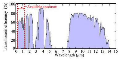
Fig. 3. Atmosphere transmission wavelength absorption (Jin and Zhou, 2019).
