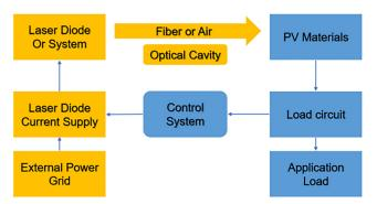
Fig. 1. Basic LPT structure. LPT, laser power transmission; PV, photovoltaics.
